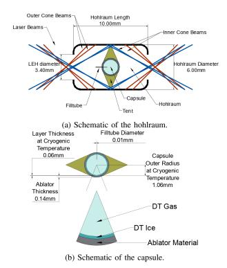
Fig. 2: Schematic of the variables corresponding to the hohlraum and capsule physical group. The dimensions in *mm* are taken as the mean dimension from the experimental dataset and they are included to give the reader an estimate.
