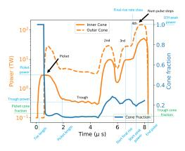
Fig. 3: Schematic of the laser power (inner and outer cone beams) and cone fraction as a function of time (laser physical group).
