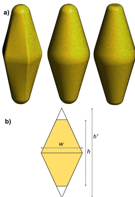
**Figure 1.** (a) The GNBs' models used in this work, including, from left to right the bipyramidal with pentagonal base and spherical tip (BPS), the biconical with spherical tip (BCS) and the biconical with flat tip (BCF) shapes. (b) A schematic representation of the basic geometric parameters of GNBs, with base length ( $w$ ), height ( $h$ ), and 2D projected area (in yellow) being extracted from TEM images, from which the nontruncated, ideal height ( $h'$ ) can be derived.
