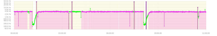
Fig. 5. A typical half-day profile of the input (green, open histogram) and recorded (magenta, shaded) trigger rate, and data acquisition errors (vertical spikes). The drop and recovery of the input trigger rate corresponds to the loss of the beam and refill, while the lack of the output trigger rate corresponds to dead time due to an error.
