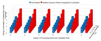
Figure 3: Energy consumption of networking equipment for nonresilient scenario and resilient scenario, without geographical constraints
