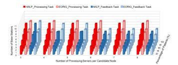
Figure 25: Number of base stations used to serve the processing and feedback tasks for the MILP model and the EORIG heuristic with different percentage of patients, for different number of processing servers per candidate node
