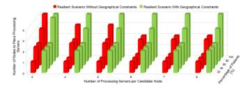
Figure 10: Number of nodes used to place processing servers for resilient scenario, without geographical constraints and resilient scenario considering geographical constraints
