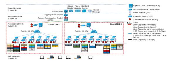
Figure 1: The resilient fog computing infrastructure under GPON access network for health monitoring applications [31]
