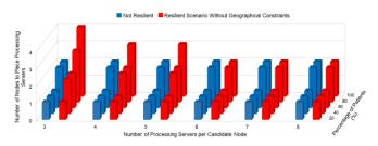
Figure 5: Number of nodes used to place processing servers for non-resilient scenario and the resilient scenario, without geographical constraints
