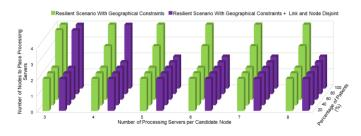
Figure 17: Number of nodes used to place the processing servers for the resilient scenario considering the geographical constraints and the resilient scenario with geographical constraints and link and node disjoint resilience
