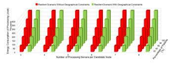
Figure 13: Energy consumption of processing for resilient scenario without geographical constraints and resilient scenario considering geographical constraints
