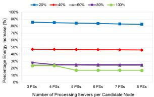
Figure 18: Percentage energy penalty of networking equipment for the resilient scenario considering the geographical constraints and link and node disjoint resilience compared to the resilient scenario considering the geographical constraints
