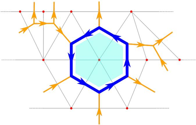
FIG. 1. Sketch of a gauge plaquette on a typical 2D CDT triangulation. For simplicity, we have considered a plaquette around a vertex with zero curvature, i.e.,  $n_b = 6$ . The direction of gauge links not belonging to the plaquette has been drawn according to the convention adopted in our code, i.e., from left to right and from bottom to up. Even if drawn differently, due to the representation on a plane, all triangles in this and the following figures should be considered equilateral.
