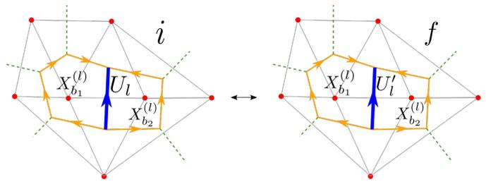
FIG. 2. Sketch of a typical gauge move, where the only difference between the initial and final state is the value of the link variable associated to the edge  $l$  (in blue) of the graph dual to the triangulation. The orientation of the link products for the staples  $X_{b_1}^{(l)}$  and  $X_{b_2}^{(l)}$  is indicated by the arrows (in the orange path).
