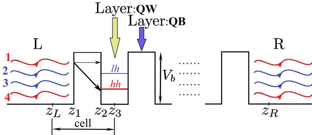
FIG. 1: (Color online). Schematic representation of quantum transport of heavy holes ( $hh$ ) and light holes ( $lh$ ) in a superlattice of  $GaAs$ - electrode ( $L$ ) /  $(AlAs/GaAs)^n$  /  $GaAs$ - electrode ( $R$ ), with no external fields and strains. QW(QB) stands for quantum well(barrier), respectively.
