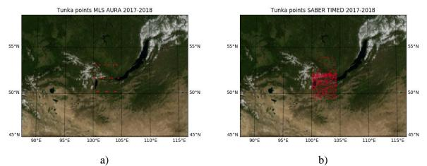
Fig1. Accumulated points of measurements in a certain area from different satellite instruments: a) MLS Aura, b) SABER TIMED
