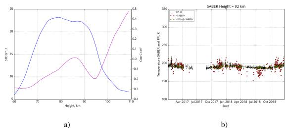
Fig. 5 Results of SABER TIMED and IFP visualizations: a) error function S (a, b) as "STDErr" purple color and Pearson correlation coefficient "CorrCoeff" blue color in relation to height, b) seasonal temperature behavior: red - temperatures obtained by SABER TIMED, dark - temperatures obtained by FPI, yellow - Fabry Perot temperatures averaged over a two-hour interval relative to the SABER TIMED measurement time.
