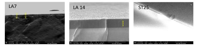
Figure S1. Cross sectional views of LA7, LA14 and ST25 (tilted at 60°) nanocomposite thin films.
