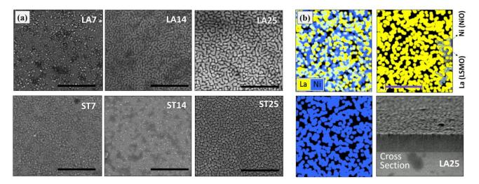
Figure 3: (a) FE-SEM micrographs of LA7/ST7, LA14/ST14 and LA25/ST25 composite thin films grown on single crystalline LAO/STO (001) substrates. (b) EDS elemental mapping of the LA25 sample, distribution of La (yellow) and Ni (blue) elements corresponding to the LSMO and NiO phases along with a cross-sectional view. Horizontal scale-bar in the image is equivalent to 500 nm.
