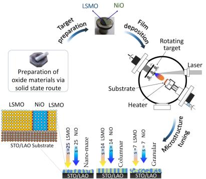
Figure 1: Scheme for the fabrication of LSMO:NiO nano-composite thin films with different resulting microstructures based nano-granular, nano columnar and nano-maze nanostructures, tuned by the growth parameter: number of laser shots 's' [(LSMO)s/(NiO)s]t(50 minutes).
