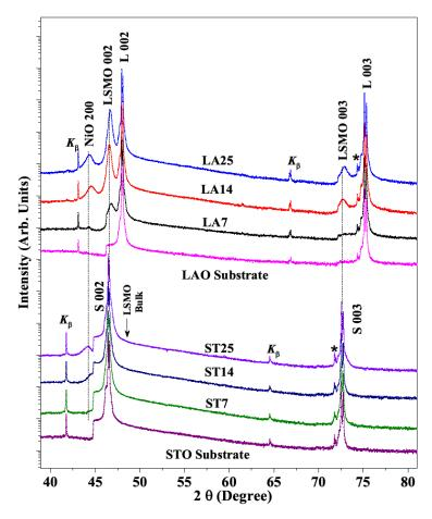
Figure 2:  $\theta$ -2 $\theta$  X-ray diffractograms of LSMO:NiO composite thin films LA7/ST7, LA14/ST14 and LA25/ST25 along with those of the reference (001) oriented single crystalline LAO(L)/STO(S) substrates. The peak represented by the asterisk arises due to the K $\alpha$  satellite interference.<sup>38</sup>
