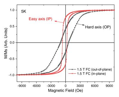
Figure S2. In-plane and out-of-plane 1.5 Tesla field cooled magnetic hysteresis behavior of LA14 composite thin film at 5K.
