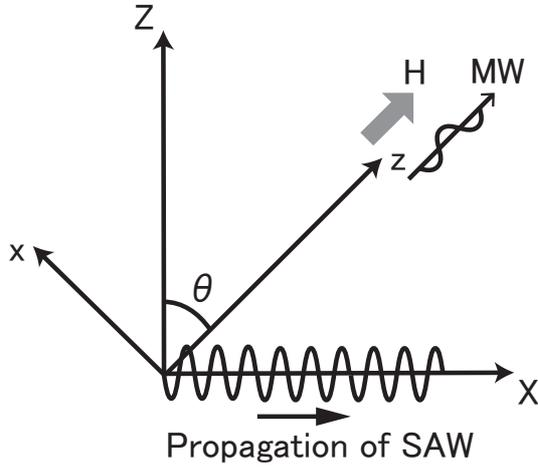
**Fig. 2.** Schematic diagram of hybrid measurement with EPR and SAW. The  $(X, Z)$  and  $(x, z)$  coordinates are set for the SAW propagating along the  $X$  axis and for the rotating static magnetic field  $H$  parallel to the  $z$  axis, respectively. The MW magnetic field oscillates along the  $x$  axis. For a silicon wafer, vacancies are distributed randomly in the  $XY$  plane of the surface layer.
