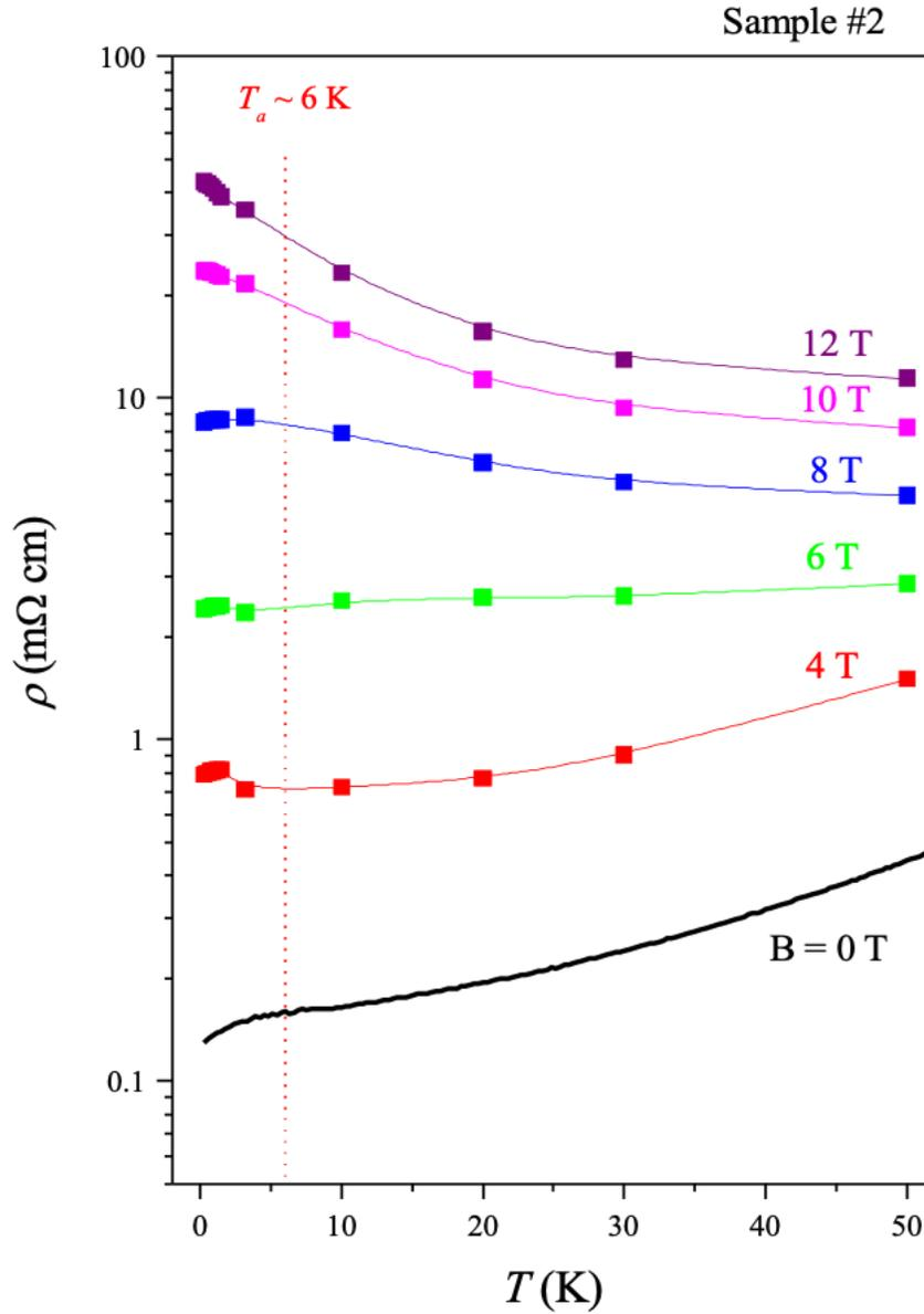
**Figure S3.**  $T$  dependence of electrical resistivity at various applied magnetic fields. Data at 0 T are measured during a  $T$  sweep, while field data are extracted from magneto-resistance (MR) data. An anomaly at  $T_a$  is seen at least up to 8 T, which greatly exceeds the reported the critical field of pressure-induced superconductivity in ZrTe<sub>5</sub>.
