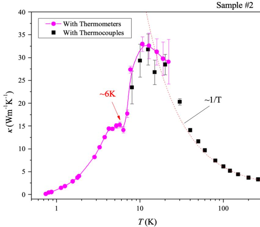
**Figure S2.** Thermal conductivity as a function of  $T$  for Sample #2. Thermometers were used because of their higher sensitivity at low temperatures due to their semiconducting nature with large negative slope of their resistance (magenta). On the other hand, thermocouples are more sensitive at higher temperatures (black). In our experiments, we observe the overlapping  $T$  range from  $\sim 10$  to  $\sim 20$  K. The dashed line (red) denotes the  $1/T$  dependence curve.
