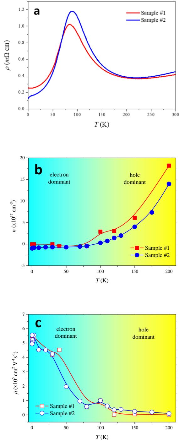
**Figure 1.** (Color Online) The  $T$ -dependent electrical resistivity  $\rho$  (a), the dominant carrier density  $n$  (b), and their mobility  $\mu$  (c) of ZrTe<sub>5</sub> single crystals. To extract the  $n$  and  $\mu$ , a two-band model was used for high  $T$  data (above 40 K), while the values at low  $T$  (below 40 K) were taken from the Hall measurement by the linear fitting method.
