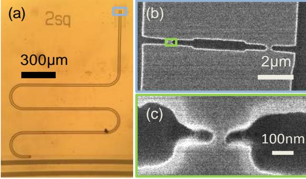
Fig. 1. Nb Dayem-bridge device. (a) Optical micrograph of the CPW meander resonator with feedline at the bottom of the image; (b) Helium FIB image of the highlighted region in (a) showing the SQUID loop; (c) Helium FIB image of the highlighted region in (b) showing a single Dayem bridge. In all images the Nb is bright and the exposed Si substrate is dark. Further details are given in [10].
