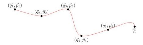
FIG. 1. A discretization of a path into N = 6 position vectors and N - 1 = 5 momentum vectors.
