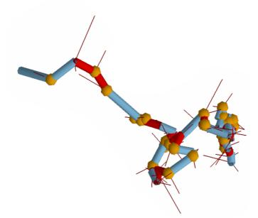
Figure 5 Typical snapshot of polymer chain embedded in the percolated network for Z=40,  $\varphi_c=0.5$ , and  $\lambda = 3.3$ . Thin lines are the partner segments connected at cross-links and slip-links. The yellow ball shows the cross-links. The segments in blue and red carry the tension below and above a specific critical value.
