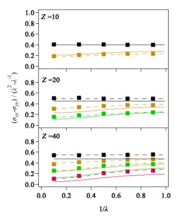
**Figure 3** Mooney-Rivlin plot of elongational stress for Z=40, 20 and 10, from top to bottom at  $\varphi_c=1$  (black), 0.5 (orange), 0.25 (green), and 0.1 (magenta) in comparison to the theory by Ball et al. <sup>11)</sup> Solid and broken curves are the theoretical predictions with the parameters determined from  $\varphi_{ac}$  and  $\varphi_{as}$ , and optimized for the best fit, respectively. The sliding parameter is fixed at  $\eta = 0.2$ .
