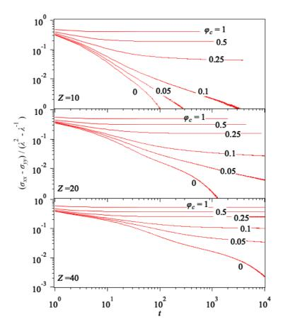
Figure 2 Stress relaxation after an instantaneous uniaxial stretch with the Hencky strain of 3 for various nominal cross-linking fraction  $\varphi_c$ . The molecular weight of the prepolymer is 10, 20, and 40 from top to bottom.
