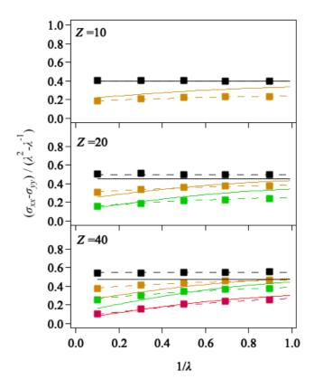
**Figure 4** Mooney-Rivlin plot of elongational stress for Z=40, 20 and 10, from top to bottom at  $\varphi_c=1$  (black), 0.5 (orange), 0.25 (green) and 0.1 (magenta) in comparison to the theory by Rubinstein and Panyukov<sup>12</sup>). Solid and broken curves are the theoretical predictions with
