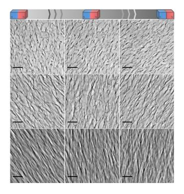
**Figure 4**: Sequential frames taken from the movies 1, 2 and 3 showing the motion of the cilia in response to the movement of an external magnet. From top to bottom: cilia obtained from 0.005 wt%, 0.01 wt% and 0.05 wt%  $\gamma$ -Fe<sub>2</sub>O<sub>3</sub>@PAmPh, respectively. Scale bars 20  $\mu$ m.
