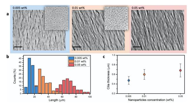
**Figure 3:** Effect of nanoparticles concentration on the dimensions of the formed cilia. (a) Optical microscopy images of the cilia prepared from 0.005 wt%, 0.01 wt% and 0.05 wt%  $\gamma$ -Fe<sub>2</sub>O<sub>3</sub>@PAmPh. Scale bars 20  $\mu$ m. The insets show a top view of the filaments in upright position. Measured cilia size in each case: (b) Cilia length distribution, (c) Average cilia thickness (diameter).
