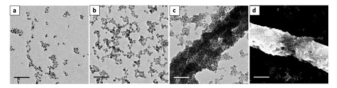
**Figure 2:** Steps of the assembly process towards the formation of filaments. TEM images of (a) magnetic  $\gamma$ -Fe<sub>2</sub>O<sub>3</sub>@PAmPh dispersion below LCST, (b)  $\gamma$ -Fe<sub>2</sub>O<sub>3</sub>@PAmPh heated to 37°C, (c)  $\gamma$ -Fe<sub>2</sub>O<sub>3</sub>@PAmPh aligned and assembled in a magnetic field during heating, Scale bars 100 nm. (d) SEM image of a filament exhibiting local voids in the structure, Scale bar300 nm.
