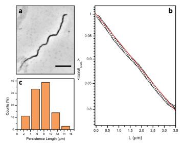
**Figure 5:** Analysis of the persistence length of the magnetic filaments. (a) Optical microscopy image of an isolated filament adsorbed on glass used to trace its contour length. Scale bar 10  $\mu$ m. (b) A representative plot of cos  $\vartheta_{s,s+L}$  as a function of the separation L along the contour and the respective exponential fitting. (c) Persistence length distribution obtained from the fitting of individual magnetic filaments.
