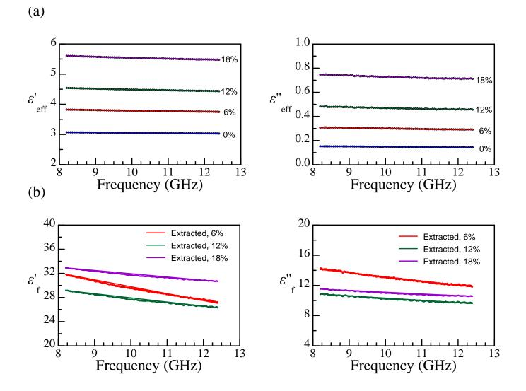
**Figure 1.** (a) The measured (effective) complex permittivity versus frequency and (b) the extracted complex permittivity of the Fe<sub>3</sub>O<sub>4</sub> nanoparticles using the Looyenga model (Eq. (1)).
