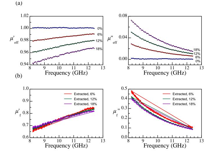
**Figure 2.** (a) The measured (effective) complex permeability versus frequency and (b) the extracted complex permeability of the Fe<sub>3</sub>O<sub>4</sub> nanoparticles using the linearly proportional model (Eq. (2)).
