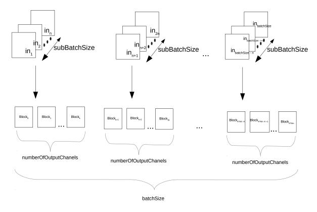
Figure 1: The total number of thread's block using to perform convolution for a single layer
