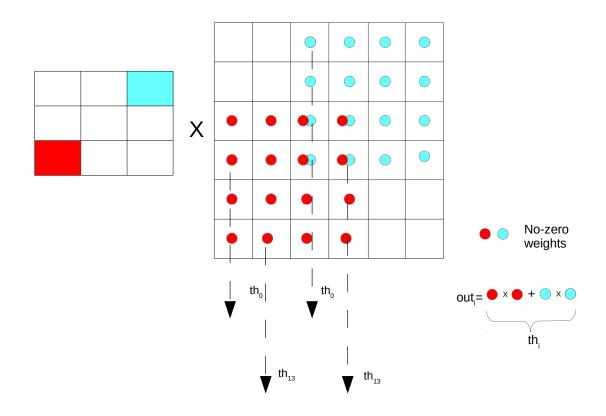
Figure 2: Calculating convolution using a sparse operation
