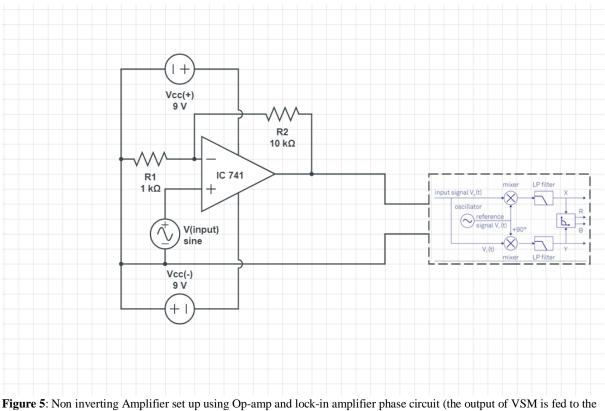
**Figure 5**: Non inverting Amplifier set up using Op-amp and lock-in amplifier phase circuit (the output of VSM is fed to the amplifier)
