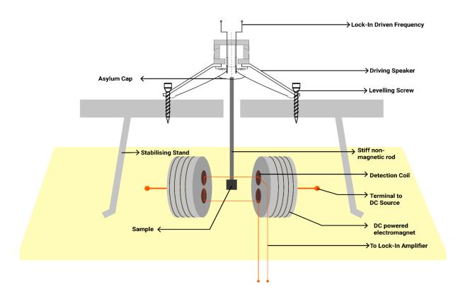
Figure 1: Schematics of homemade vibrating sample magnetometer (VSM) set up
