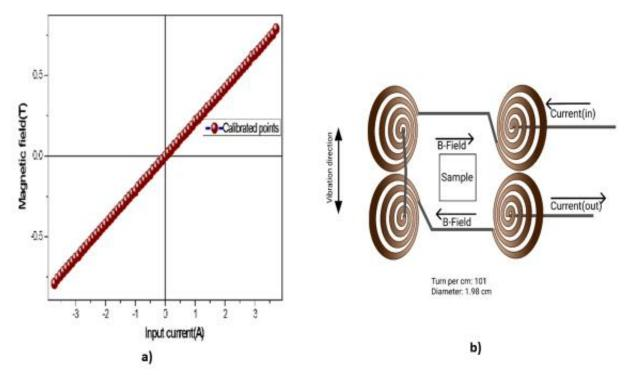
**Figure 3**: a) Variation of the magnetic field with DC current supplied for all values of current -4 A to 4 A b) Spiral detection coils and its specified orientation to obtain maximum induced voltage
