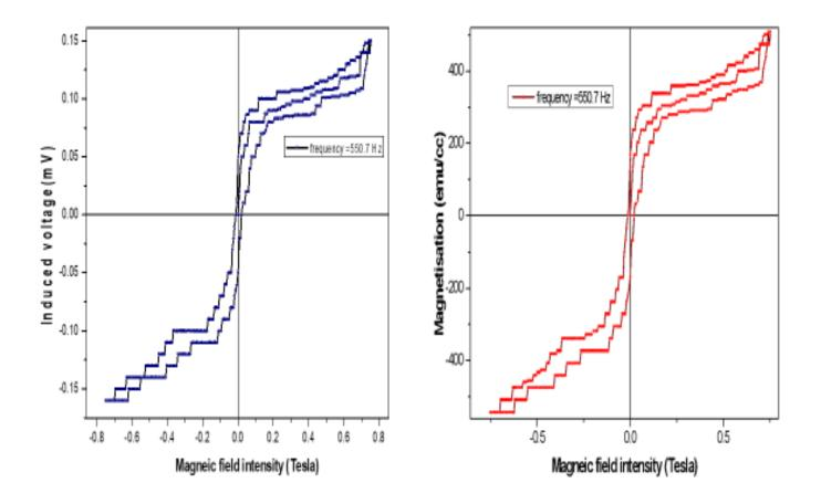
**Figure 4**: (a)Variation of induced voltage with respect to the magnetic field intensity for Nickel (99%) (b)Variation of magnetization with respect to the magnetic field intensity for Nickel (99%)
