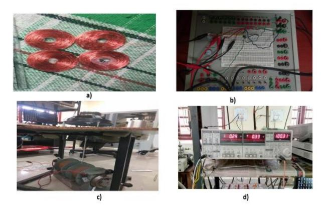
**Figure 2**: a)Detection coils used in vibrating sample magnetometer (VSM) set up b) Snap of the non-inverting Amplifier for booster circuit c) Homemade Vibrating sample magnetometer set up d) Stanford model SR830 Lock-in amplifier
