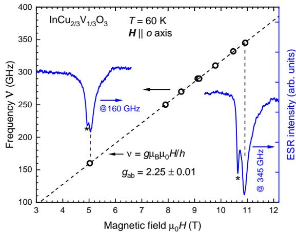
FIG. 2. Frequency  $\nu$  versus magnetic field  $H$  dependence of the ESR signal of the oriented powder sample of  $\text{InCu}_{2/3}\text{V}_{1/3}\text{O}_3$  measured at  $T = 60$  K with  $\mathbf{H} \parallel \mathbf{o}$  axis (open circles). A corresponding fit is shown as dashed line. Exemplary ESR signals are shown for frequencies of 160 and 345 GHz. The asterisk labels a small additional peak presumably due to  $\text{Cu}^{2+}$  spins at defect sites.
