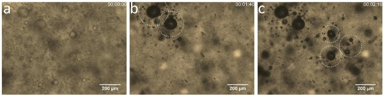
Figure 9 – Optical microscopy images showing the reopening pore clusters during drying of the sample D50-5NaCl at 110°C.
