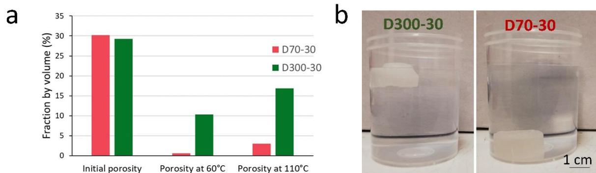
Figure 6 – a) Characteristics of the dried thick samples with different pore sizes; b) a photograph of the dried samples demonstrating flotation (D300-30) and sinking (D70-30) in pure water.
