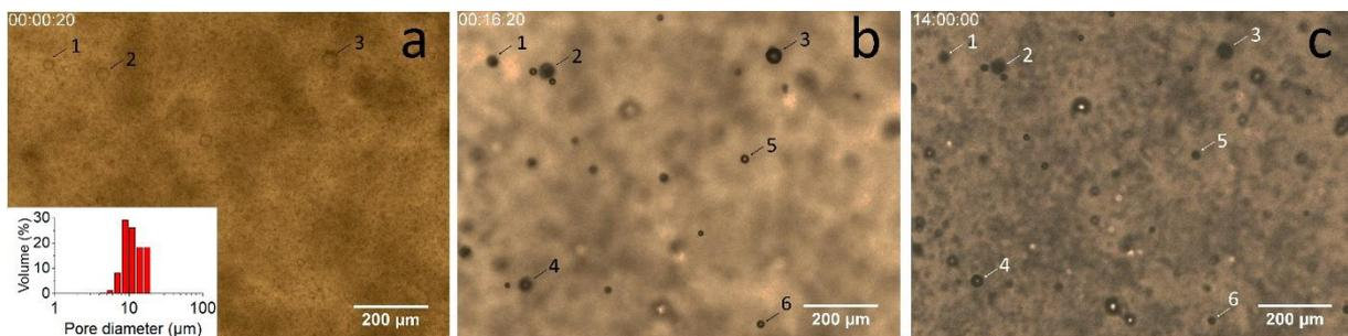
*Figure 3 – Optical microscopy images of the D10-5 sample during drying at 60°C: a) initial state (small pores are poorly visible); b) state after 16 min of drying; c) state after 16 hours of drying. The insert on the image a) shows the pore diameter distribution in the initial state. Some clearly identified pores are labeled with numbers.*
