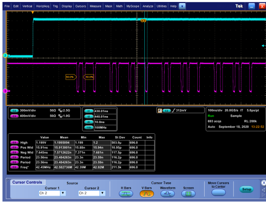
Fig. 17. Waveform of two SMA from the FPGA. The blue waveform is an enable signal to enable 500 inferences. The pink waveform is the results of the inferences. The oscilloscope is running at infinite persistence mode. The sharp edge of the pink signal shows that the operations are always at fixed latency. The minimum width of the pink pulse of 8 ns shows that the hardware is able to refresh the inference at a speed of 125 MHz. The 16 clock cycles difference between the enable and the first valid inference result shows that the latency is 128 ns.
