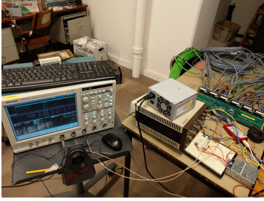
Fig. 16. This picture shows the hardware performance evaluation platform, on the right is the BEC with TTIM powered by redundant power supply, on the left side one can see the DPO7000 oscilloscope displaying the waveform of the two signals transferred through two SMA cables to the TTIM.
