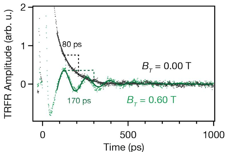
**Figure S6.** A comparison of TRFR traces collected with and without an applied magnetic field at  $T = 4.5$  K from Figure 2a in the main text. Solid lines show fits to the data using eq. 1, while the dashed lines illustrate the time for the sample to decay to  $1/e$  amplitude, 80 ps for  $B_T = 0.00$  and 170 ps for  $B_T = 0.60$ . Under an applied magnetic field, the nuclear spin bath becomes polarized, suppressing inhomogeneous magnetic (hyperfine) fields that accelerate dephasing.
