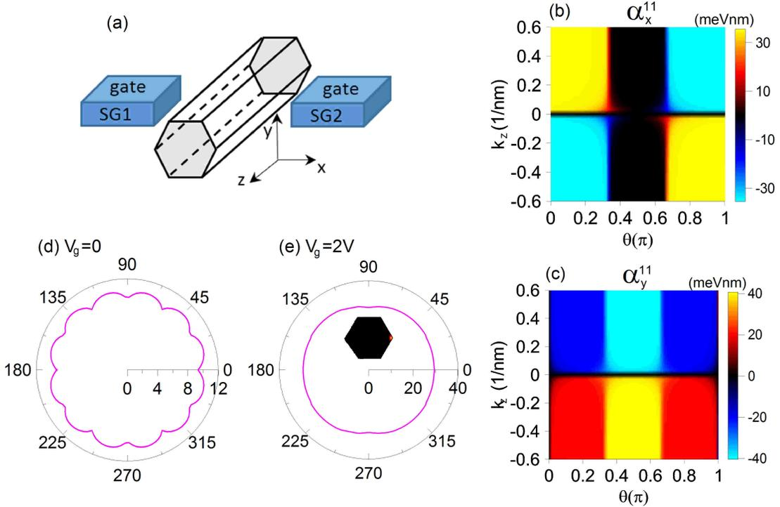
FIG. 14. (a) Schematic illustration of the experimental setup. (b,c) The  $x$ - and  $y$ - component of the intra-subband SO coupling  $\alpha_i^{11}$  as a function of the angle  $\theta$  and the wave vector  $k_z$ . The magnetic field is rotated in the  $x - y$  plane. (d,e) The angular dependence of the total SO constant,  $\alpha_{tot}$ . Results for  $B = 0.1$  T and  $\phi = \pi/2$ .
