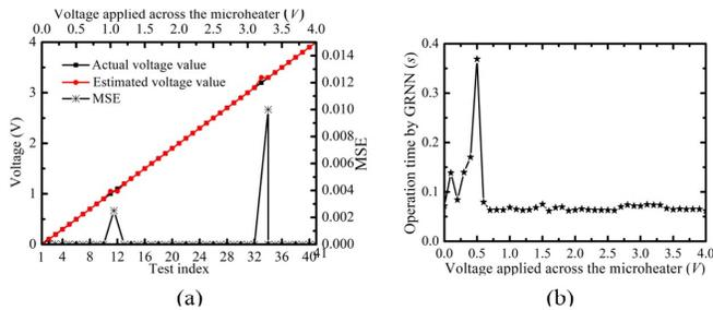
Figure 7. All the intensity samples in the spectra at  $1500 \text{ nm} \leq \lambda \leq 1620 \text{ nm}$  are used to form the original data, and the GRNN algorithm is adopted to develop the predictive model. (a) The comparison between the estimated values of the voltage and their corresponding actual values versus voltage applied across the microheater, and MSE versus voltage applied across the microheater. (b) Operation time by the GRNN versus voltage applied across the microheater.
