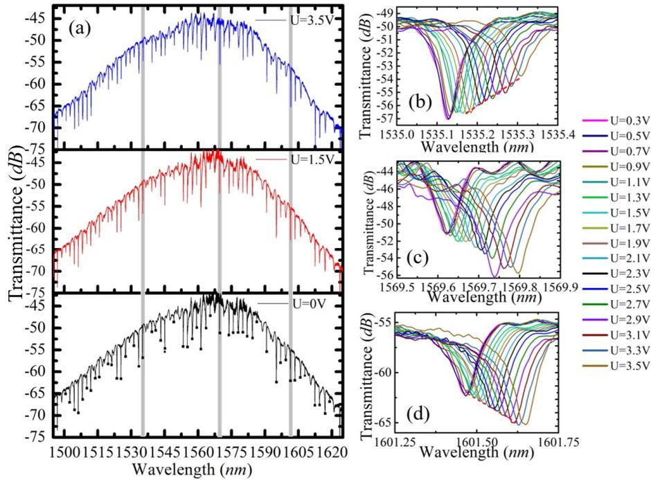
Figure 3. (a) With the micro-heater driven by various DC voltages ( $U=0, 1.5, 3.5$  V), the experimentally measured transmission spectra of the SIMRR sensor excited by a broadband laser source, and the transmission dips near 1535.2 nm, 1569.7 nm and 1601.5 nm are indicated by the shadows. When the DC voltages applied across the micro-heater is changed from 0.3 V to 3.5 V with the step size of 0.2 V, the experimental transmission spectra near 1535.2 nm (b), 1569.7 nm (c), and 1601.5 nm (d).
