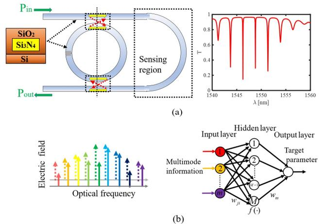
Figure 1. The proposed multimode sensing mechanism. (a) Structural diagram of a SIMRR-based sensor design and typical amplitude transmittance of a SIMRR. (b) An ANN assisted multimode sensing information fusion for predicting the target parameter.
