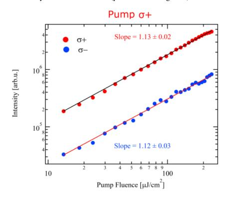
**Figure S5.** Power dependence measurements acquired under circular polarized ( $\sigma$ +) excitation with the same angle (i.e.,  $\Theta_p = 11^\circ$ ) as in Fig.3 of the main text, but with higher excitation energy ( $E_p = 2.0598eV$ ), as shown by the dotted line P2 in Fig. S4b. The data are plotted in a log-log scale and fit with a power law of the form y(x) = kx<sup>n</sup>, where n represents the slope of the lines used in the fittings.
