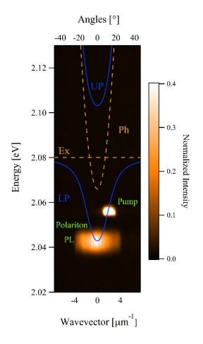
Figure S3. Energy and wavevector resolved emission intensity under resonant excitation, showing both the pump laser ("Pump"), which is incident at an angle  $\theta_p = 11^\circ$ , and the exciton-polariton photoluminescence (PL) emission. The intensity of the pump laser is saturated for illustrative purposes.
