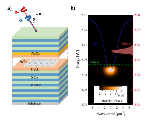
**Fig.2-(a)** Schematic of the microcavity sample, composed of two (Nb<sub>2</sub>O<sub>5</sub>/SiO<sub>2</sub>) DBRs and a WS<sub>2</sub> monolayer sandwiched between two protective (HSQ and Al<sub>2</sub>O<sub>3</sub>) layers (see SI for details). The
