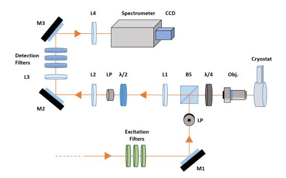
Figure S7. Sketch of the optical setup used in the experiments. List of the optical components: M1, M2, and M3 are mirrors; LPs are linear polarizers; BS is a non-polarizing beam splitter;  $\lambda/4$  is a quarter-wave plate; Obj. is the objective used for excitation and collection, with 40x magnification and 0.65 numerical aperture; L1, L2, L3, and L4 are convex lenses;  $\lambda/2$  and LP are respectively the quarter-wave plate and the linear polarizer used to measure the Stokes parameters.
