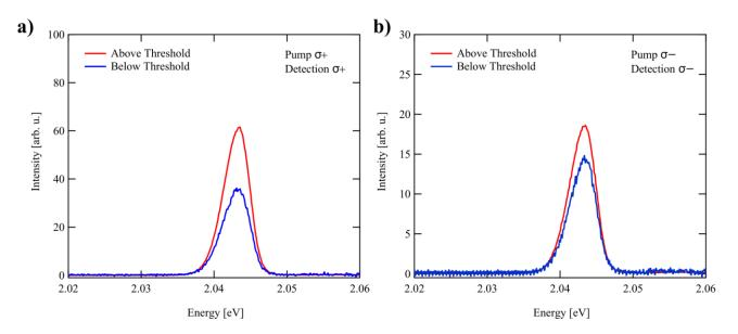
**Figure S6.** Energy resolved intensity profiles of the polariton emission, co-polarized with the excitation pump, in K (**a**) and K' (**b**) valley, normalized by the excitation fluences below (blue trace) and above (red traces) the bosonic stimulation threshold.
