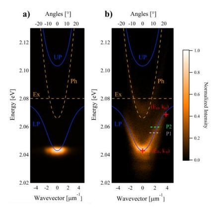
**Figure S4.** Energy and wavevector resolved emission intensity under, **a**) resonant and **b**) nonresonant excitation. The yellow dotted lines represent the theoretical exciton (Ex) and photon (Ph) dispersion, while the blue lines represent the lower (LP) and upper (UP) polariton branches. The red crosses in
