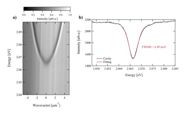
**Figure S2. a)** Experimental white light reflectivity measurements of the MC sample used in the experiment. **b)** Intensity profile extracted along the vertical axis in a), from 2.048eV to 2.085eV and  $|\mathbf{k}| < 0.5 \mu \text{m} - 1$ . The red line represents the inverse Gaussian fitting used to calculate the FWHM and the resonance of the photonic mode of the microcavity.
