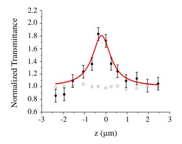
**Figure S1**. *z*-scan normalized transmittance traces of the GSA (full dots) probed with a QCL frequency comb operating at 10% duty cycle, compared with the z-scan normalized transmittance traces of the Si/SiO<sub>2</sub> substrate (empty dots). The error bars correspond to the uncertainty interval on the measured normalized transmittance. The dashed lines are fits of the normalized transmittance T(z) using the following equation
