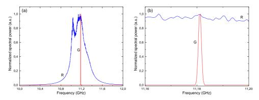
Figure S3. (a) Simulated beatnote power spectrum for the bare laser (blue trace) (sample R) and for the device with the GSA (red trace) (sample G). The parameters employed to describe the simulated systems are summarized in Table I. (b) Zoom on the intermode betanote of sample G. A further reduction of the intermode beatnote linewidth is expected for increased simulation times, beyond the actual capabilities of the employed computer.
