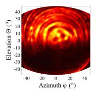
**Figure S2.** Far-field intensity profile of the double metal THz QCL comb measured whilst driving the QCL with a current I = 800mA at 15 K, and placing the pyroelectric detector at 6 cm from the laser facet.
