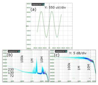
Figure 2: Experimental charcteristics from the Class-A push-push configuration of the 'N3' SQUID array. (a) Flux response. (b) Flux noise spectrum, in vertical units of  $n\Phi_0/Hz^{1/2}$ . (c) Frequency response obtained with pseudorandom flux noise excitation shows -3 dB bandwidth of 13 MHz.
