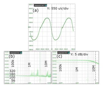
Figure 3: Experimental characteristics from the Class B push-push configuration of the 'N3' chip. (a) Flux response. (b) Flux noise spectrum, in vertical units of  $n\Phi_0/Hz^{1/2}$ . (c) Frequency response obtained with pseudorandom flux noise excitation shows -3 dB bandwidth of 12.5 MHz.
