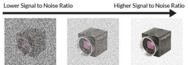
Figure 2: Effect of Signal to Noise Ratio (SNR) on Image Quality. A reduced SNR can result in less analysable content making vision based safety system defunct in low light applications.
