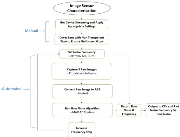
Figure 3: Image Sensor Characterisation Flowchart
