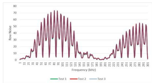
Figure 4: Characterisation Repeatability. Omnivision OV7955 image sensor performance characterisation in response to electrical noise carried out 3 times and overlaid to demonstrate repeatability.
