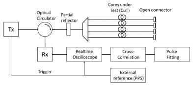
Fig. 1 Schematic of the C-OTDR laboratory setup to simultaneously measure four cores of a multi-core fiber.
