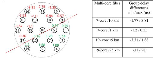
Fig. 3 Left: Differential group delay variations with respect to the center core of the 5-km, 19-core fiber; right: minimum and maximum group delay differences of different multi-core fibers.
