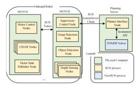
Fig. 2. Architecture for a distributed robot-planning system (adapted from [10]
