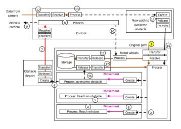
Fig. 10. Adding an obstacle to the window-opening robot.
