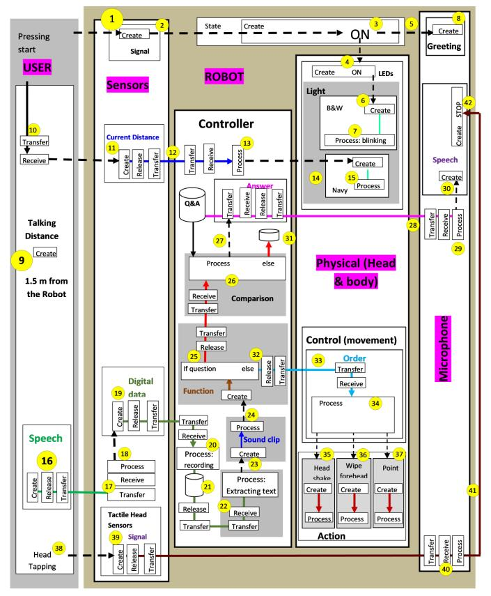
Fig. 16. TM model of the NAO robot's architecture.
