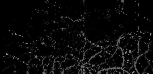
Figure 2. Sample image of the image processing applied to each image, based on the original shown in Fig. 1c. Extreme pixels with brightness values I \in [0, 255] are exponentially enhanced, \tilde{I} = \exp[|I - 127|/127] , focusing attention on the portions of the image that represent interparticle forces.
