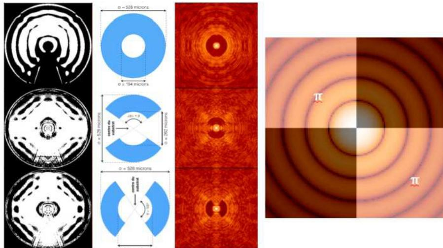
Figure 2. On the left: the Shaped Pupil coronagraphic masks. On the right: the Four Quadrant Phase Mask.
