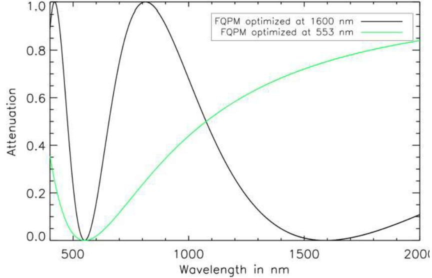
Figure 4. Comparison between theoretical PSF attenuation as a function of wavelength for a FQPM optimized at  $1.6\mu\text{m}$  and a FQPM optimized at 553nm. The former can cancel a star at 550nm (sharp), but its high sensitivity to the bandwidth makes it worse in performance with respect to the latter at the end.
