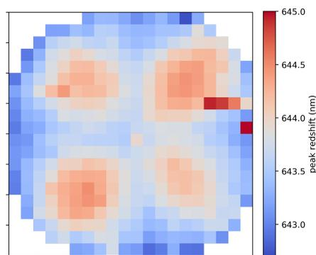
**Fig. S4:** Peak redshift map of neutral exciton on a single ZnPc measured with a metallic tip at  $V_{\text{DC}} = -3.1$  V. The redshifts are derived from the dataset presented in Fig. 2A.
