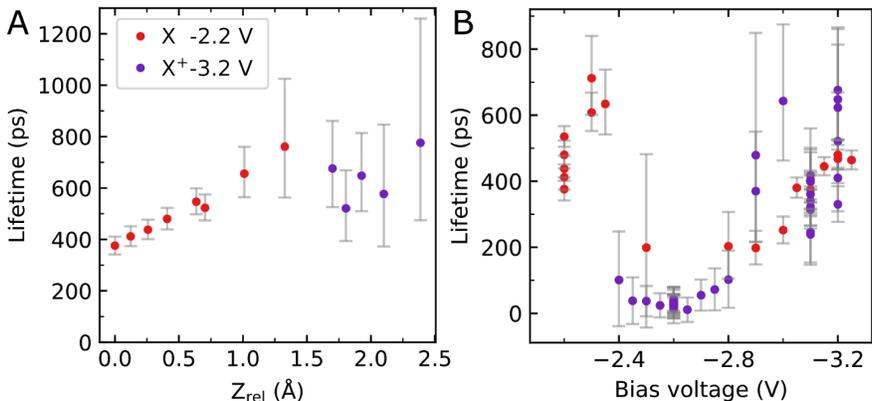
**Figure 3. Dependence of lifetimes on picocavity size and bias voltage.** (A) Lifetime of neutral exciton (red) and trion (purple) as a function of tip-molecule relative distance ( $Z_{rel}$ ). (B) Lifetime of neutral exciton (red) and trion (purple) as a function of applied  $V_{DC}$ . A 200 MHz harmonic signal with 100 mV amplitude is used for measuring the phase shift and determination of the lifetimes. Range of  $I_t$  was 50 to 130 pA.
