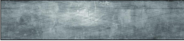
Fig. 1. Recording of the cylinder wall of a combustion engine by a line scan camera as used by Breitmeier Messtechnik GmbH (Beyerer et al. 2016)
