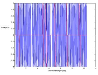
Figure 8 Effect of broken sensor ring teeth for the crank and cam position sensor signals.
