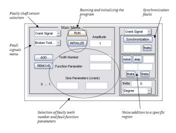
Figure 7 Control panel of graphical user interface.
