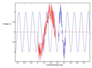
Figure 10 Close-up view of generated partially faulty crankshaft and camshaft sensor signal pulses.
