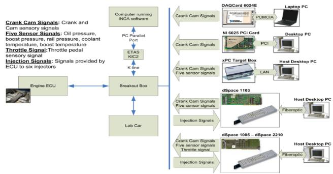
Figure 1. A general view of the hardware portion of the HiL setup showing all the hardware platforms used.
