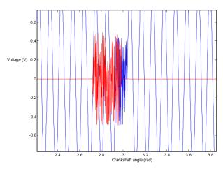
Figure 11 Close-up view of generated faulty crankshaft and camshaft sensor signal pulses.
