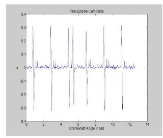
Figure 3 Real engine cam shaft sensory data.
