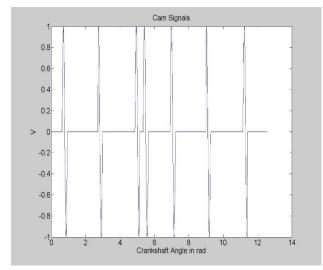
Figure 5 Generated camshaft position sensor signal.
