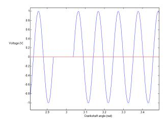
Figure 9 Close-up view of Figure 8 showing broken sensor ring tooth for the crank position sensor signal.
