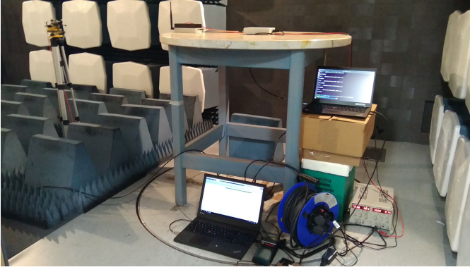
Fig. 4. Anechoic chamber setup for RF WPT experiments.
