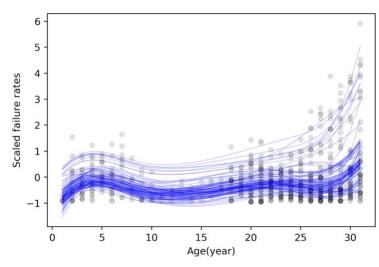
Fig. 5 is the result of HS model predicting the total lifetime failure rate of 99 ship engines. Spots are points of failure with 99 data. Considering the missing data in the early period due to warranty repair (as in section 3.1), they are bathtub-formed, as some previous literature has suggested (as in section 2.2). Among the models introduced in section 2.2, Prophet and ARIMA are selected as baseline models each for its high accuracy and popularity, respectively. We would like to
