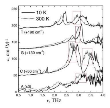
Fig. 2. Spectral dependences of the extinction ratio of (A) adenine, (C) cytosine, (G) guanine, and (T) thymine obtained at temperatures of (solid line) 10 and (dashed line) 300 K [7].
