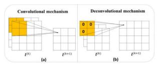
Fig. 3 (a) Convolutional and (b) deconvolutional operations.
