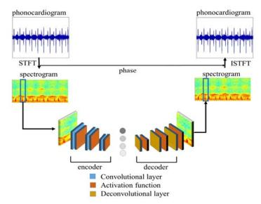
Fig. 1. The convolutional deep autoencoder (DAE(C)) architecture.
