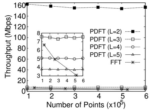
**FIGURE 8:** Throughput of FFT and the proposed PDFT algorithms for a number of points  $N = 1 \cdot 10^5, 2 \cdot 10^5, \dots, 6 \cdot 10^5$ . For FFT, only the powers of two  $2^{17} = 131072, 2^{18} = 262144$  and  $2^{19} = 524288$  are considered.
