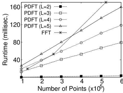
**FIGURE 7:** Runtime of FFT and the proposed PDFT algorithms for a number of points  $N = 1 \cdot 10^5, 2 \cdot 10^5, \dots, 6 \cdot 10^5$ . For FFT, only the powers of two  $2^{17} = 131072, 2^{18} = 262144$  and  $2^{19} = 524288$  are considered.
