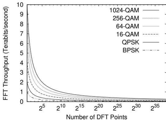
**FIGURE 1:** Asymptotic throughput of the FFT algorithm over distinct OFDM signal mappers. As the number of points increases, complexity grows faster than the number of modulated bits irrespective of the chosen mapper.
