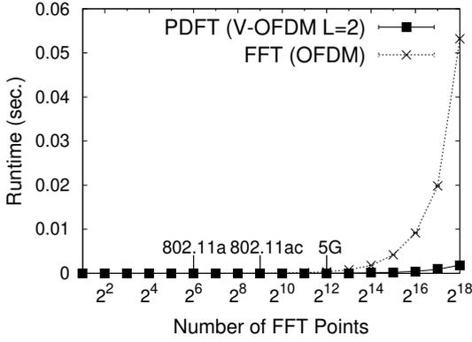
FIGURE 3: FFT vs. PDFT (proposed): Simulation runtime.
