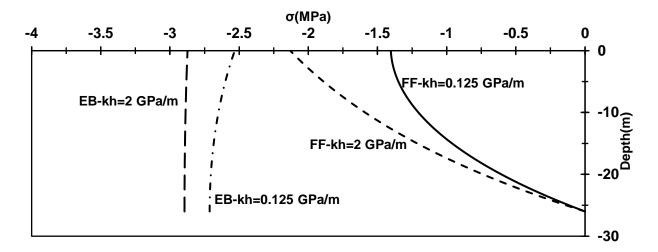
Figure 7. Thermo-mechanical axial stress of fully floating (FF) and end bearing (EB) energy piles under loading scenario (*ii*), F = -1000 kN and  $\Delta T = +10$  °C,  $k_h = 0.125$  GPa/m and  $k_h = 2$  GPa/m
