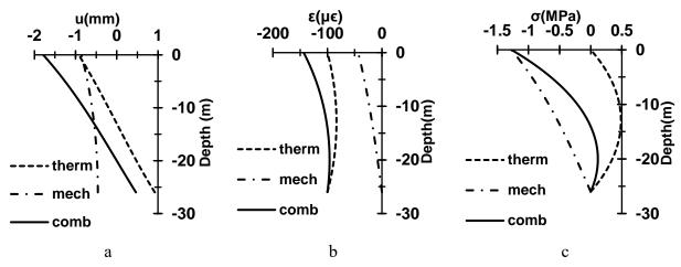
Figure 2. a) Displacement, (b) strain, and (c) stress in a fully floating energy pile subjected to thermo-mechanical load scenario (*i*), F = -1M N and  $\Delta T = -10$  °C,  $k_h = 0$
