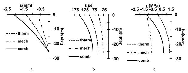
Figure 3. a) Displacement, (b) strain, and (c) stress in an end bearing energy pile subjected to thermo-mechanical load scenario (*i*), F = -1000 kN and  $\Delta T = -10$  °C,  $k_h = 0$
