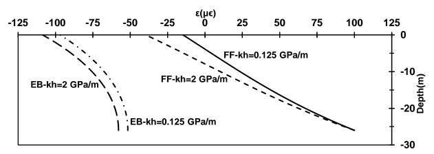
Figure 6. Thermo-mechanical axial strain of fully floating (FF) and end bearing (EB) energy piles under load scenario (*ii*), F = -1000 kN and  $\Delta T = +10$  °C,  $k_h = 0.125$  GPa/m and  $k_h = 2$  GPa/m
