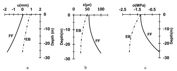
Figure 4. a) Displacement, (b) strain, and (c) stress in fully floating (FF) and end bearing (EB) energy piles subjected to thermo-mechanical load scenario (*ii*), F = -1000 kN and  $\Delta T = +10$  °C,  $k_h = 0$
