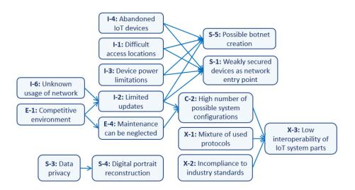
Fig. 1. Typical consequences among specific features and challenges having an impact on quality characteristics of IoT systems.
