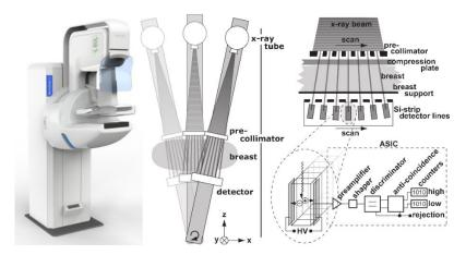
Fig. 1. Left: Photograph and schematic of the Philips MicroDose S0 prototype spectral tomosynthesis system. **Right:** The image receptor and electronics.
