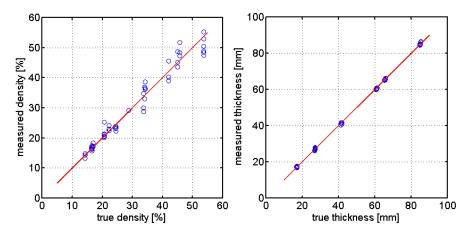
**Fig. 2.** Breast density (left) and thickness (right) as a function of ground truth from 57 phantom configurations. One-to-one lines are included for reference (red solid lines).
