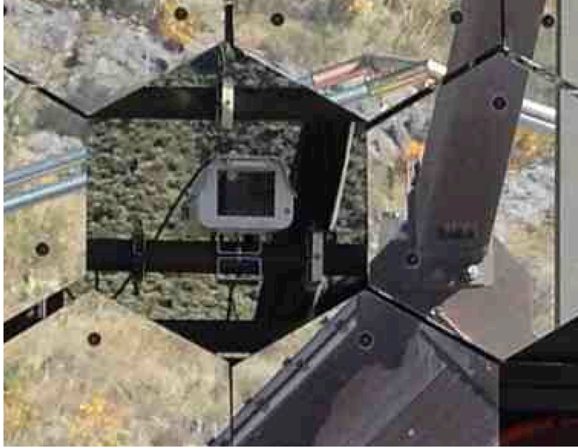
Figure 2: A photograph of the Pelco box containing the SBIG camera and control computer mounted near the centre of a VERITAS reflector, in place of one of the mirror facets.
