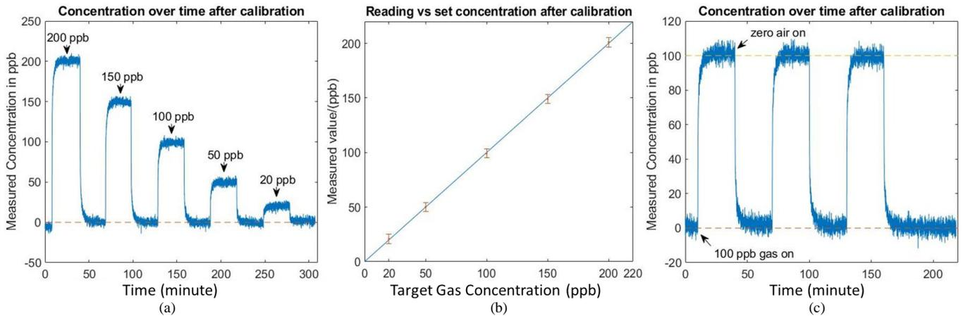
Fig. 5. Sensor calibration results: a) the sensor response to different concentrations of  $\text{NO}_2$ , at 200 ppb, 150 ppb, 100 ppb, 50 ppb, 20 ppb with low hysteresis and a LLOD of 10 ppb; b) the sensor readings on the y axis with respect to the  $\text{NO}_2$  concentrations generated by the gas generator show good linearity and zero offset; c) repeated on-off test to ensure baseline drift is not an issue.
