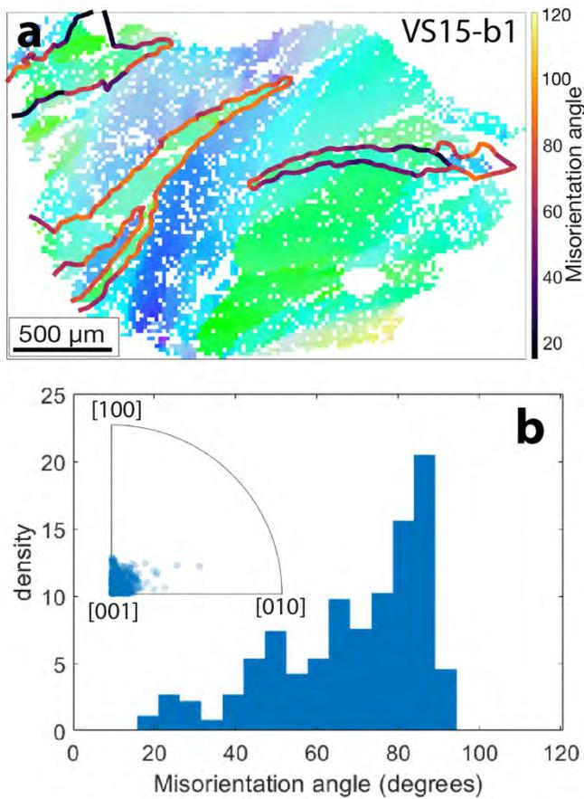
**Fig. 10.** Kinked olivine crystal in coarse-grained dunite VS15-a1 (location indicated in Fig. 9). (a) Orientation map in which kink boundaries with variable misorientation angle are highlighted. (b) Misorientation angle and axes distributions across the kink boundaries highlighted in (a).
