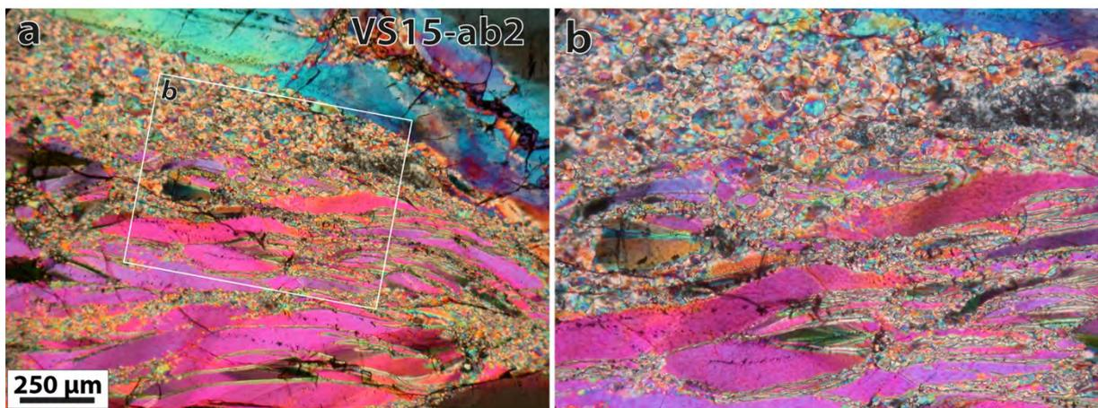
**Fig. 11.** Photomicrographs of a kinked and partially recrystallized olivine crystal in the neck region of coarse-grained dunite VS15-ab2 (location indicated in Fig. 8). Bulk extension direction is parallel to the long side of (a).
