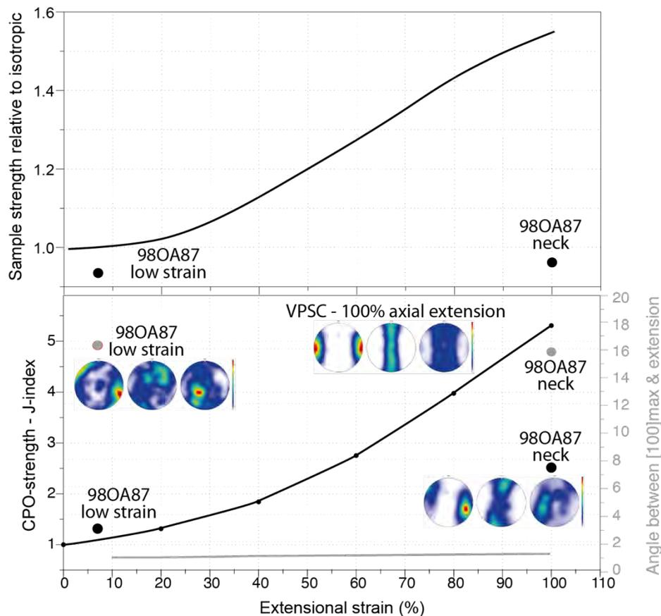
**Figure S3.** Evolution of the sample strength (top) and olivine CPO (bottom) as a function of the extensional strain predicted by the VPSC approach for an aggregate with an initially isotropic CPO subjected to axial extension (full
