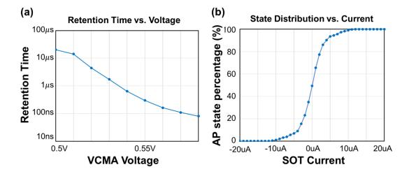
**Figure 3**. Dynamics of the VC-SOT device (a) Voltage-retention time relationship calculated from the LLG equation, showing a linear relationship in the semi-log plot; and (b) SOT induced probability bias. These relationships follow those derived in Section 2.
