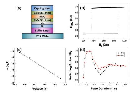
**Figure 8**. (a) Film stack of perpendicular MTJ. (b) Hysteresis loop of the MTJ. The shift in the magnetic R-H loop is due to the stray field of fixed layer. (c) Thermal stability dependence on applied voltage. (d) Switching probability of free layer with various pulse durations with the stray field compensated.
