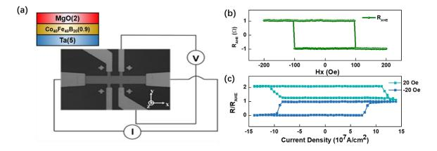
**Figure 6.** (a) Material stack of the Ta(5)/CoFeB(0.9)/MgO(2) Hall bar, and the microscope image of the 20 x 130 m Hall bar device. During the measurement, the applied current goes through the longitudinal channel of the Hall bar and the voltage is measured from the transverse channel. (b) The magnetic hysteresis loop and (c) SOT switching of the magnetization.
