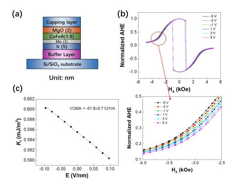
**Figure 7.** (a) Material stack for the VCMA Hall bar measurement (b) Normalized anomalous Hall resistance versus in-plane magnetic fields (hard-axis loops), under different gate voltages. We see a clear change in the anisotropy with different electric fields. (c) The extracted interfacial PMA values ( $K_i$ ) as a function of applied electric field.
