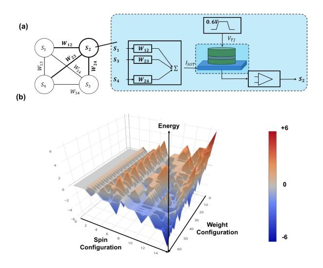
**Figure 4.** (a) Simulation setup of a 4-neuron Boltzmann machine on our MTC system. Each neuron is mapped to one MTC. For neuron *i*, its state  $S_i$  is represented by the MTJ's state, and its connected weights  $W_{ij}$  are stored in the weighted sum module. Its inputs  $x_i$  are the states of other connected neurons  $S_j$  (b) Energy landscape of the 4-neuron Boltzmann machine, with binary-coded spin configurations and weight configurations.
