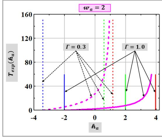
**Figure 5:** Temperature vs. system energy (Eq. (25)) at a fixed system density ( $w_a = 2.0$ ), for two values of the nonlinearity parameter ( $\Gamma = 0.3 ; 1.0$ ). Energy range for both  $\Gamma$  values is  $h_{a0} + 0.01 \cdot \Delta h_a$  to  $h_{a0} + 0.95 \cdot \Delta h_a$ . Vertical lines as in **Figure 4**. Note the very high system temperatures at the low  $\Gamma$  value.
