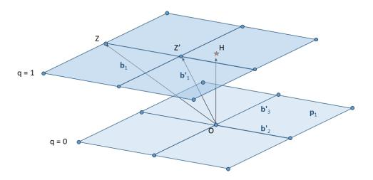
**Figure 3** Hyperplanar reduction. The lattice is "stratified" into different layers. Here only the layers q = 0 and q = 1 are represented. The vector of the layer q = 1 that should shorten/reduced is **OZ** = **b**<sub>1</sub>. The reduction is made thanks to the calculation of the point H (marked by a little orange star) which is the orthogonal projection of the origin 0 onto the layer q = 1.
