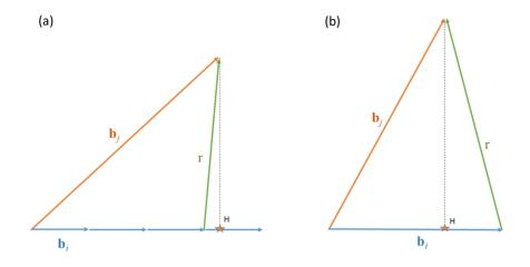
**Figure 2** Directional reduction. Case where (a)  $\lfloor q \rfloor = \left\lfloor \frac{\mathbf{b}_i^t \mathbf{b}_j}{\mathbf{b}_i^t \mathbf{b}_i} \right\rfloor = 3$ , and (b)  $\lfloor q \rfloor = 1$ . The orthogonal projection point is noted H and marked by a little orange star.
