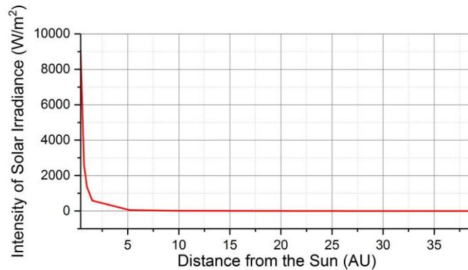
**Figure 5 Distribution of Solar Irradiance in the Solar System\***
