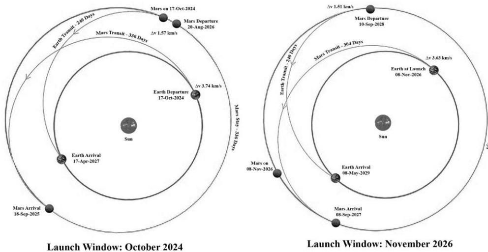
**Figure 3 Optimized Trajectory for Human Mission to Mars\***
