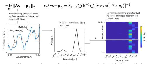
expression with a non-negative constraint using an active-set method and is implemented in the MATLAB function *lsqnonneg*. In the current study, the least squares expression was  $\min_{x} ||\mathbf{Ax} - \mathbf{\mu}_{\mathbf{b}}||_2$ , where  $\mathbf{\mu}_{\mathbf{b}}$  is the depth-dependent backscattering spectra extracted from experiment data and  $\mathbf{Ax}$  is the backscattering spectra from Mie theory, Fig. 4.
