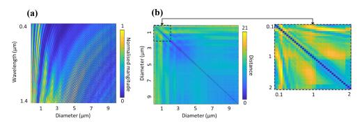
Fig. 6: (a) Backscattering spectra for polystyrene microspheres diameters 0.1 to  $10 \,\mu\text{m}$  analyzed across a wavelength range of 0.4 to 1.4  $\mu\text{m}$  and (b) the corresponding distance matrix showing that shorter wavelength and broader bandwidth light sources can improve solution stability by increasing the Euclidean distance and, in doing so, decreasing the coefficient matrix condition number.
